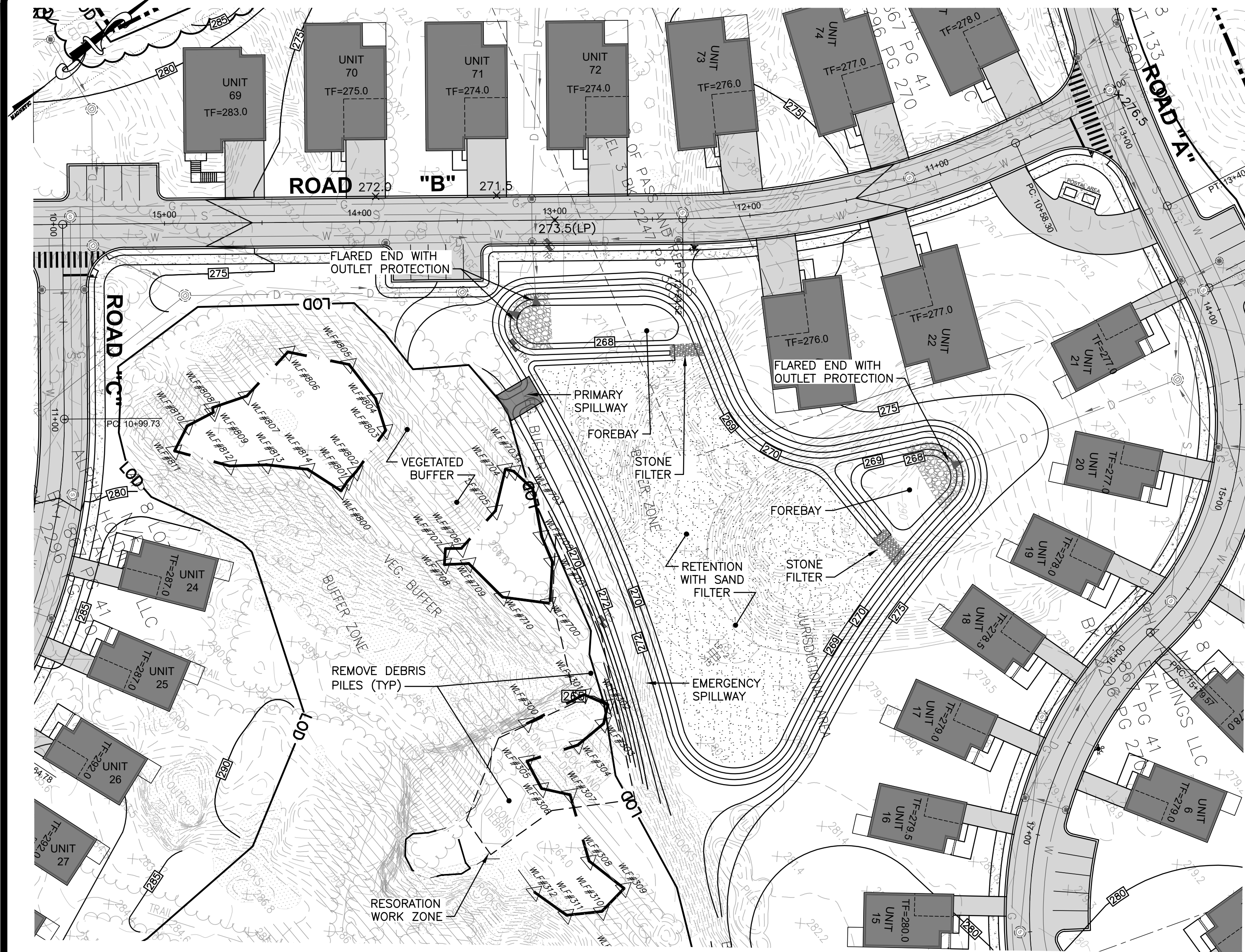
BMP-1 INFILTRATION BASIN
