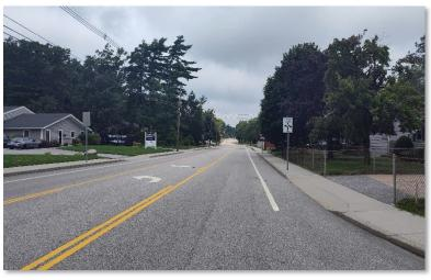
yellow median turn lane markings with turn arrows delinate the median area, and solid white markings define the shoulder area that is an extension of, and marked as a dedicated bike lane. In this area concrete sidewalks are provided along both sides of the road and there are several high visibility crosswalks with solar powered RRFB's, crossing Arnold Road that link residential neighborhoods to the east and west. These features can be seen in the above photograph looking north from Larch Drive.
