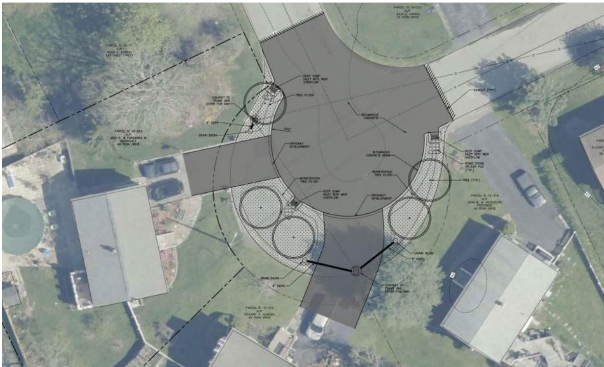
Figure 16: Partial cul-de-sac pavement removal and GSI project example in Warren, RI
