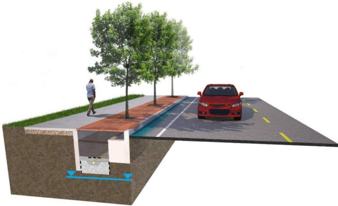
Tree box filters next to roadway
