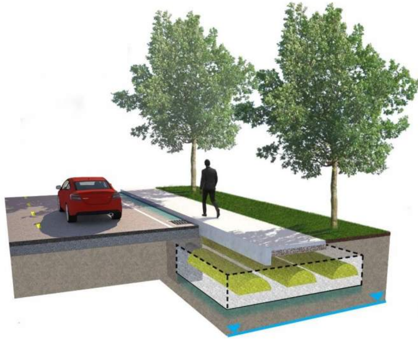
Figure 18: Subsurface infiltration chambers beneath sidewalk
