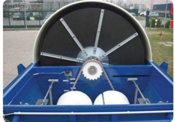
Internal view of the RBC and cloth media drum filters
