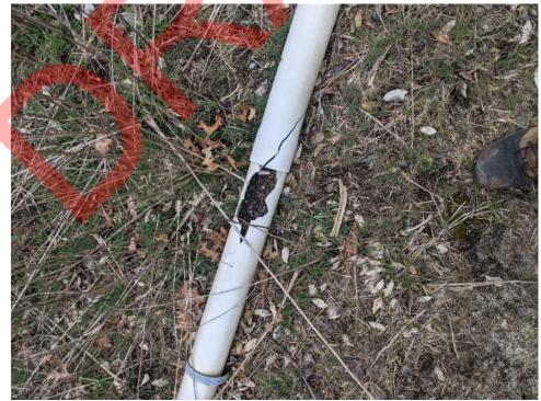
Figure 3: Cracked Sand Bed Effluent Distribution Piping
