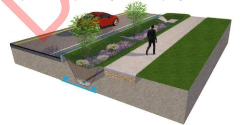
Figure 13: Bioswales between roadway and sidewalk or private property
