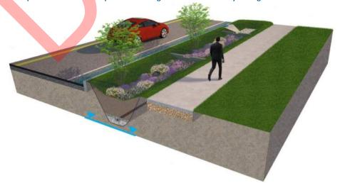
Figure 13: Bioswales between roadway and sidewalk or private property
